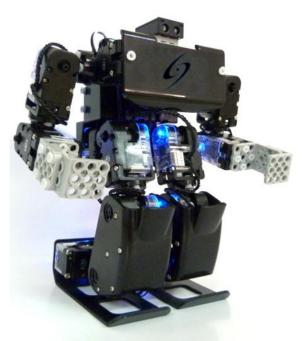
LIMBOT includes all the latest technologies available in the Humanoids field (16 DOF, proximity sensors, sound sensors, USB connectivity and Android App for remote control)
